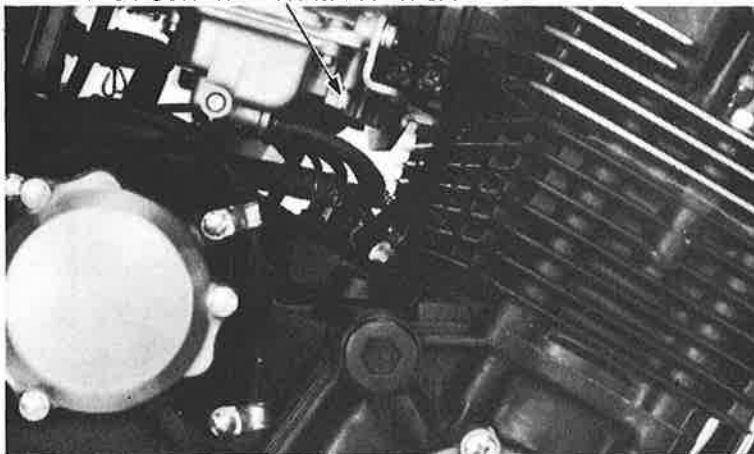
PILOT SCREW WITH LIMITER CAP
