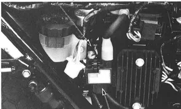
STARTER RELAY SWITCH
