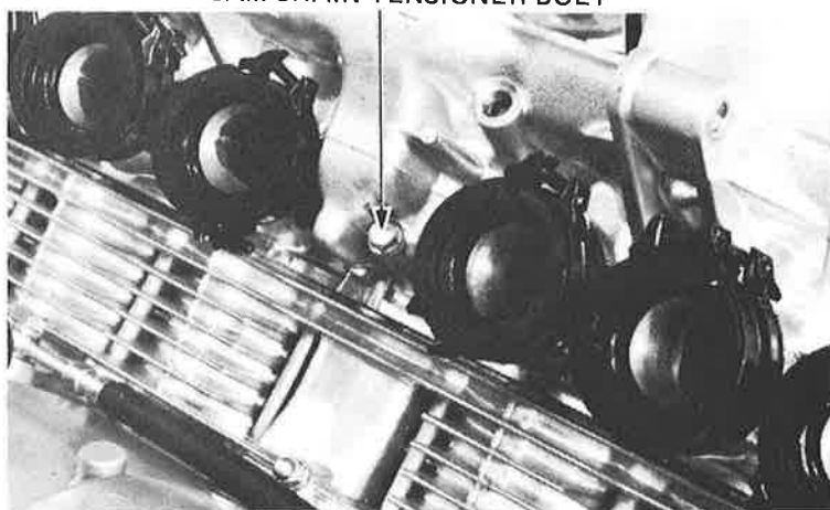
CAM CHAIN TENSIONER BOLT
