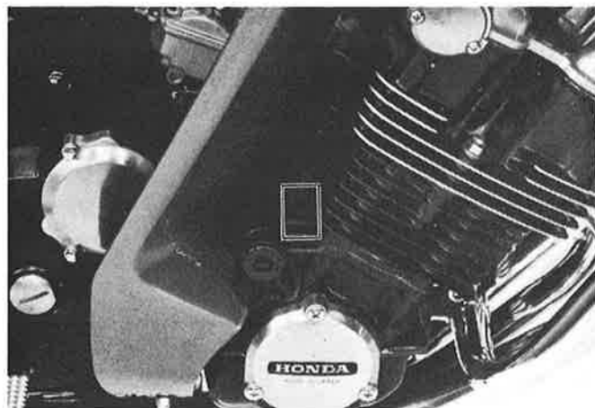
The engine serial number is stamped on the top of the crankcase.
