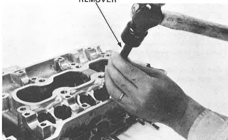
VALVE GUIDE REMOVER
