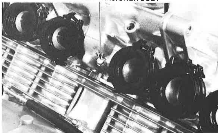
CAM CHAIN TENSIONER BOLT
