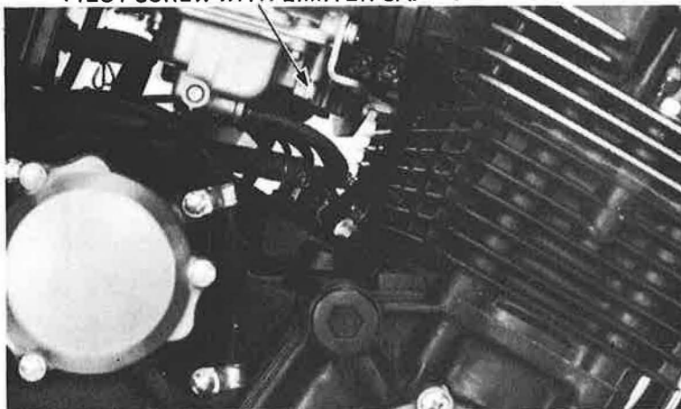
PILOT SCREW WITH LIMITER CAP
