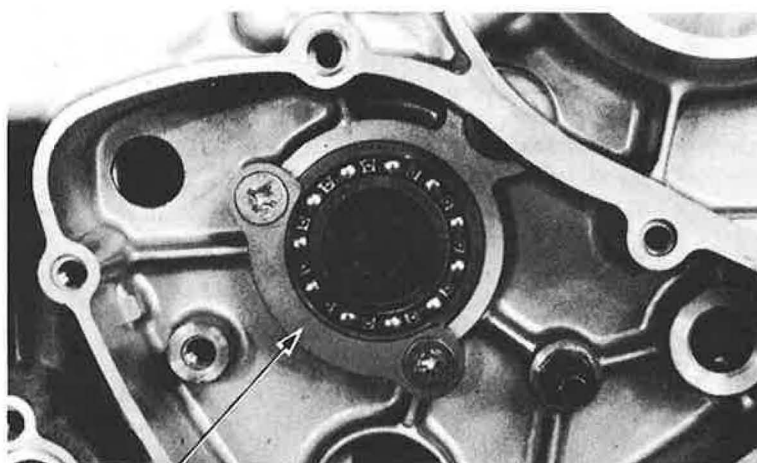
BEARING STOPPER PLATE
