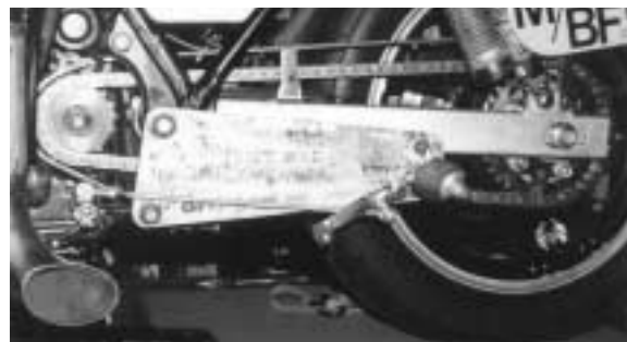
Rear sets in place
