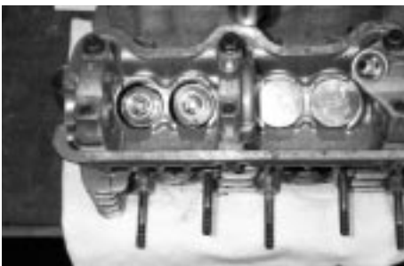
Head ground for exhaust lobe clearance
