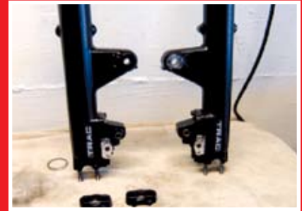
Newly painted fork bodies, ready to reinstall
