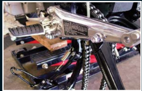
The left side foot peg bracket must be installed at same time the center stand goes on due to the fact that the through bolt goes in from the left side. Notice newly polished foot peg bracket.
