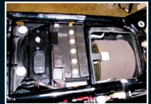
New battery and cleaned up air filter installed. The air box was treated with back to black, and looks like new again.
