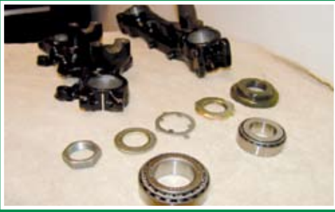
Newly painted fork bodies, ready to reinstall
