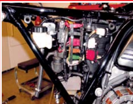
Cleaned up electrical components are re-assembled in the exact way they were from the factory. This is a case where good photos taken before disassembly come in handy so that you get back in the correct order.
