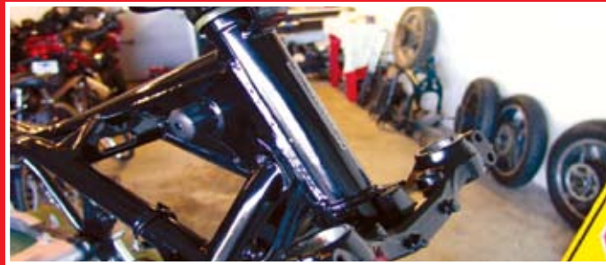
Reassembled and ready for the fork tubes
