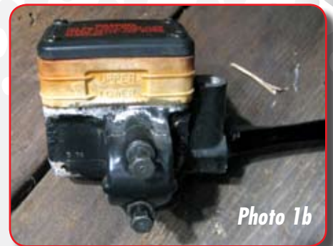
Photo 1a and 1b: A crusty seized up master brake cylinder as removed from a rusty crusty CBX which has been standing for a long time.
