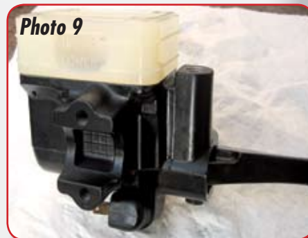
Assembly showing lever and brake light switch installed.
