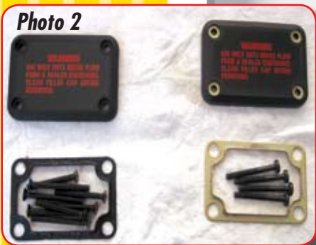
The difference between an aftermarket cap and an original one, for the aftermarket cap, the metal (very rusty) reinforcement plate has been painted black.
