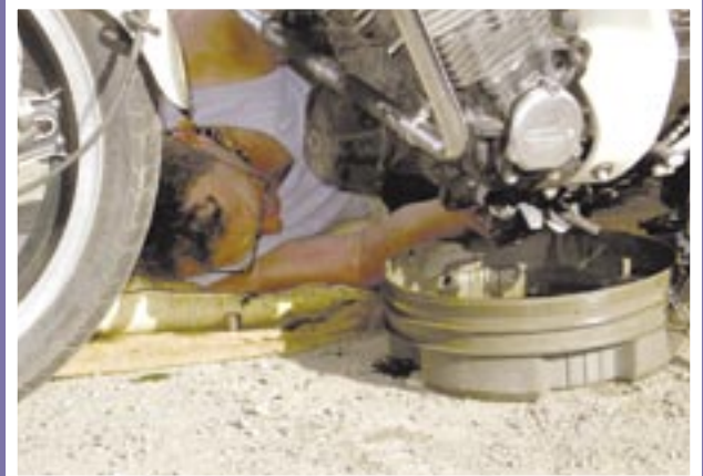
Draining oil to check for pin.
