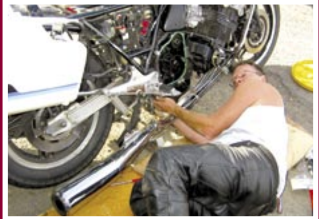
Noel removing the mufflers.
