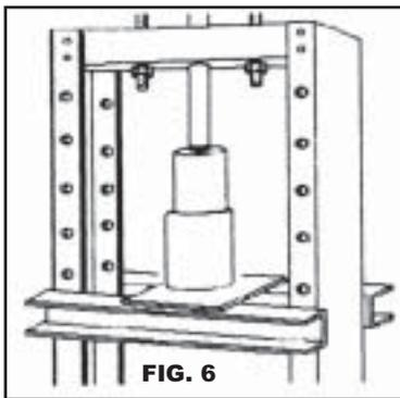
to gently drive the seal down into the case. Press the seal in until it *just* clears the circlip groove, and no further. This is important! Pushing too far will distort the shock outer case, as will also trying
