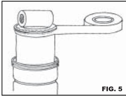
to install it with a hammer. Don't make either mistake. Put the shock back in the vise and install the circlip and dust boot, then reinstall the shock into the bike and air it up.
