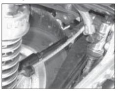
To modify the stock arm it must be cut in half and a piece welded in the middle. I welded 3/4-inch in mine but it is not quite long enough. The next tire change I will be adding another 1/2-inch.
