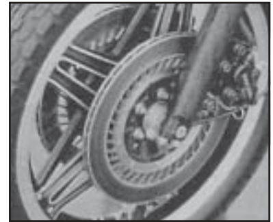
Ventilated discs with double piston caliper
