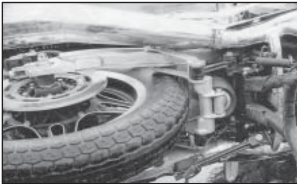
new rear wheel guidance: ProLink makes it possible with leverage
