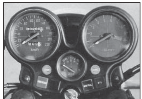
The instruments, tach, speedo and voltmeter are clear; also the idiot lights. Speedometer error: 10%
